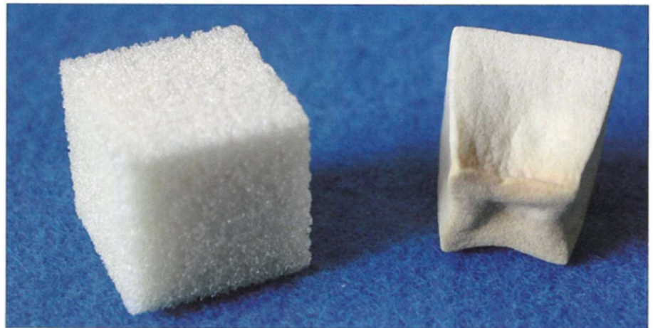
Figure 14. Specimen before water absorption (left) und deformation after water absorption (right)
